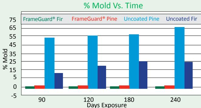
After one year and 76.3" of rainfall, there was significantly less growth of mold on corresponding samples of FrameGuard® wood. Weather-shielded samples of FrameGuard® wood had virtually no mold after the year's test.
