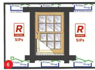
6 Apply sealant behind window flanges and install windows.
