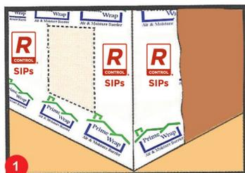
1 Start with lowest course, 2-3 feet from a corner. Secure Prime Wrap housewrap firmly in place by fastening it every 12” to 18” along the vertical studs using large-headed or plastic cap nail or 1” crown staples.
