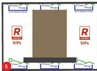
5 Temporarily tape header flap up to expose nail base material. Install the sill flashing over the housewrap.
