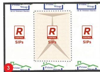
3 Make and inverted Y cut in the housewrap at rough opening. Then cut straight across the top and make diagonal cuts from the top corners to create header flap.
