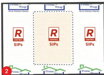
2 Continue to unroll the Prime Wrap tightly around the structure - covering all door and window openings. While nailing or stapling make sure the fabric is taut against the exterior wall and not sagging. Seal all seams, tears, and cuts with Prime Wrap Sheathing Tape.
