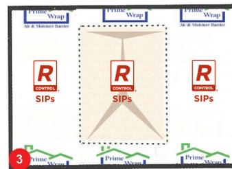
3 Make and inverted Y cut in the housewrap at rough opening. Then cut straight across the top and make diagonal cuts from the top corners to create header flap.
