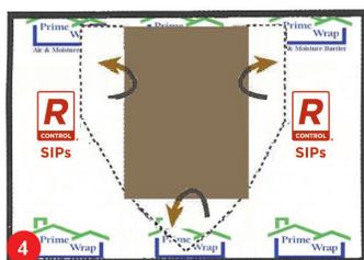
4 Fold the flaps in through the opening at the two sides and the sill and fasten them inside with staples set about every 6 inches.
