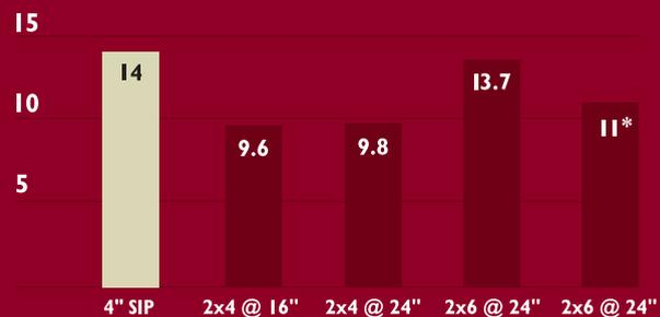
**SIP walls trounce conventional fiberglass methods in "whole-wall R-value" comparisons.**
