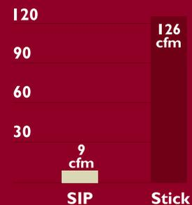
**Recent tests at Oak Ridge National Laboratory (ORNL) confirm the super airtightness of SIP construction.**
