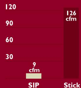
**Recent tests at Oak Ridge National Laboratory (ORNL) confirm the super airtightness of SIP construction.**
