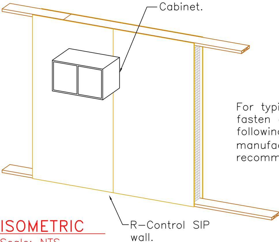
For typical cabinet loadings fasten cabinet to panels following cabinet manufacturer's recommendations.
