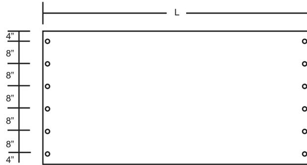
Connection patterns for single span condition
