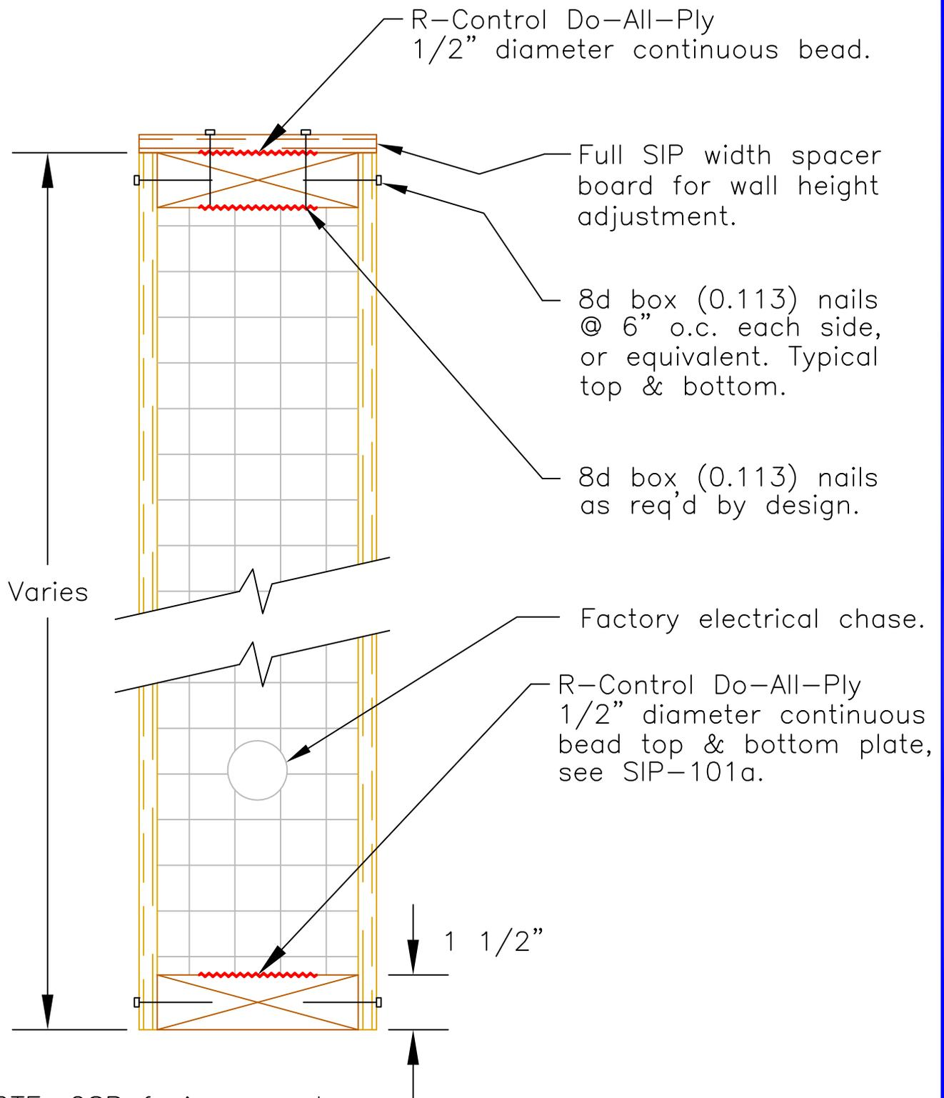
NOTE: OSB facings must be fully supported by foundation system.
