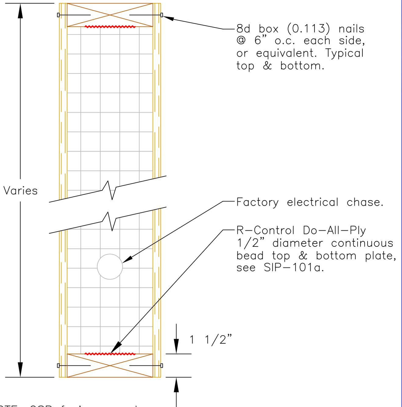
NOTE: OSB facings must be fully supported by foundation system.
