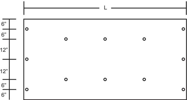
*Connection patterns for four span condition*
