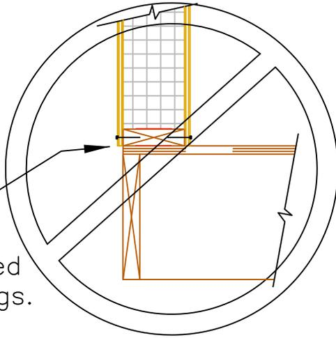
Don't have OSB facings and untreated plates in direct contact with concrete.
