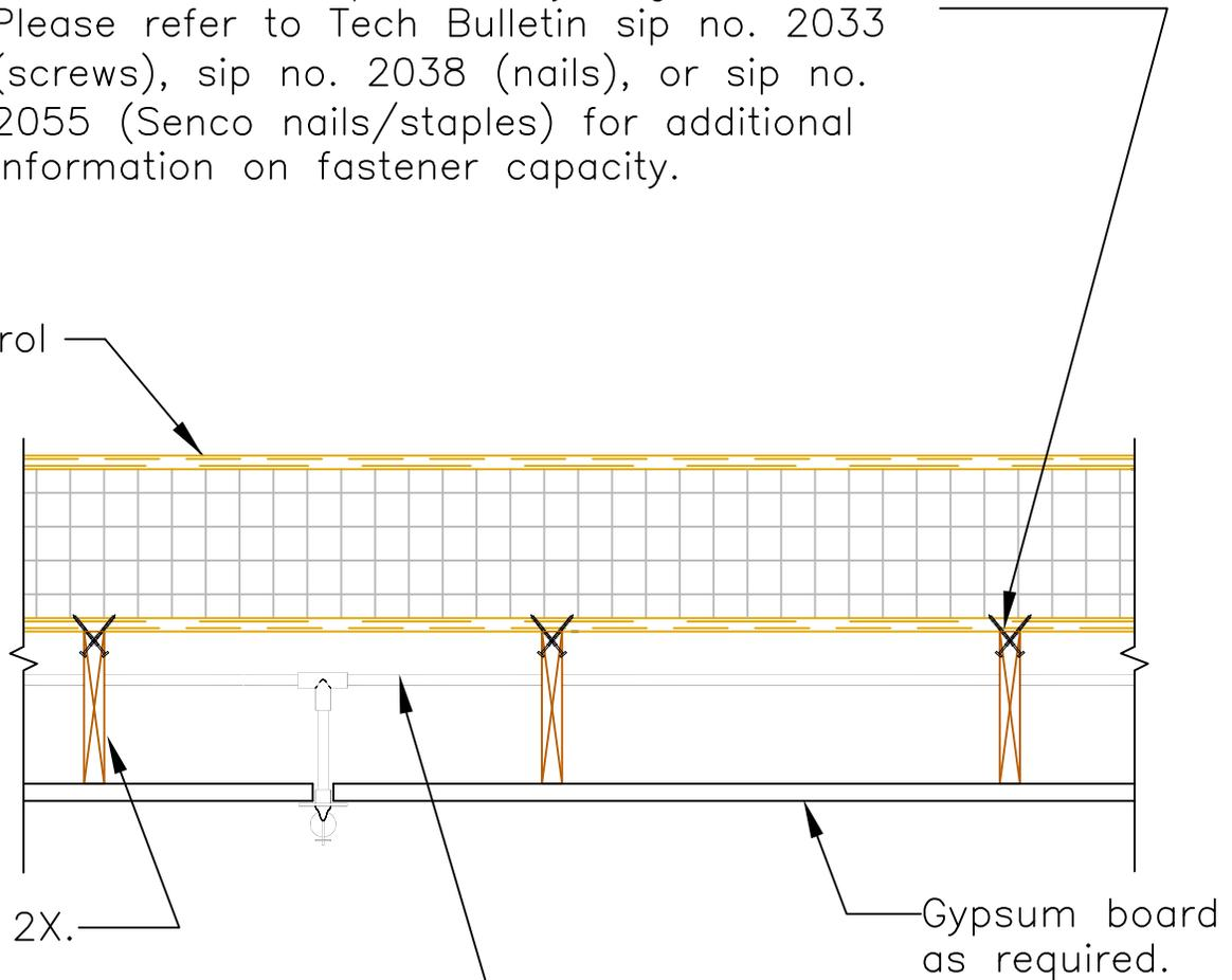
Note: 2X to be sized as required for cavity depth. 2X may be placed flat against R-Control SIP.
