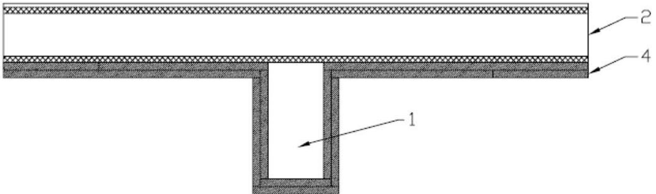
1. Wood Beam - Min 4-1/2 in. wide by 9-1/2 in. deep size wood beam spaced in accordance with manufacturer's specifications.
