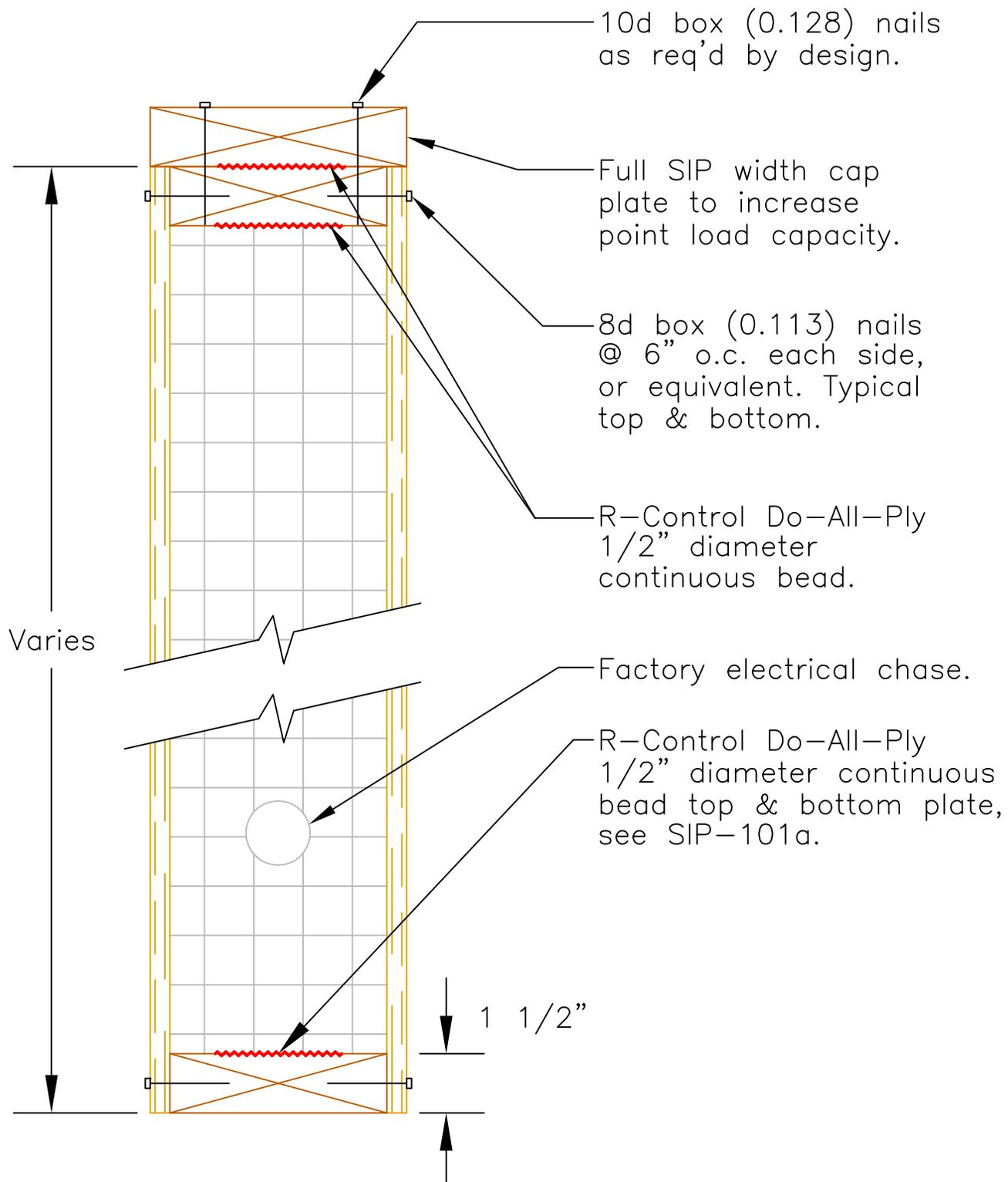
NOTE: OSB facings must be fully supported by floor/foundation system.
