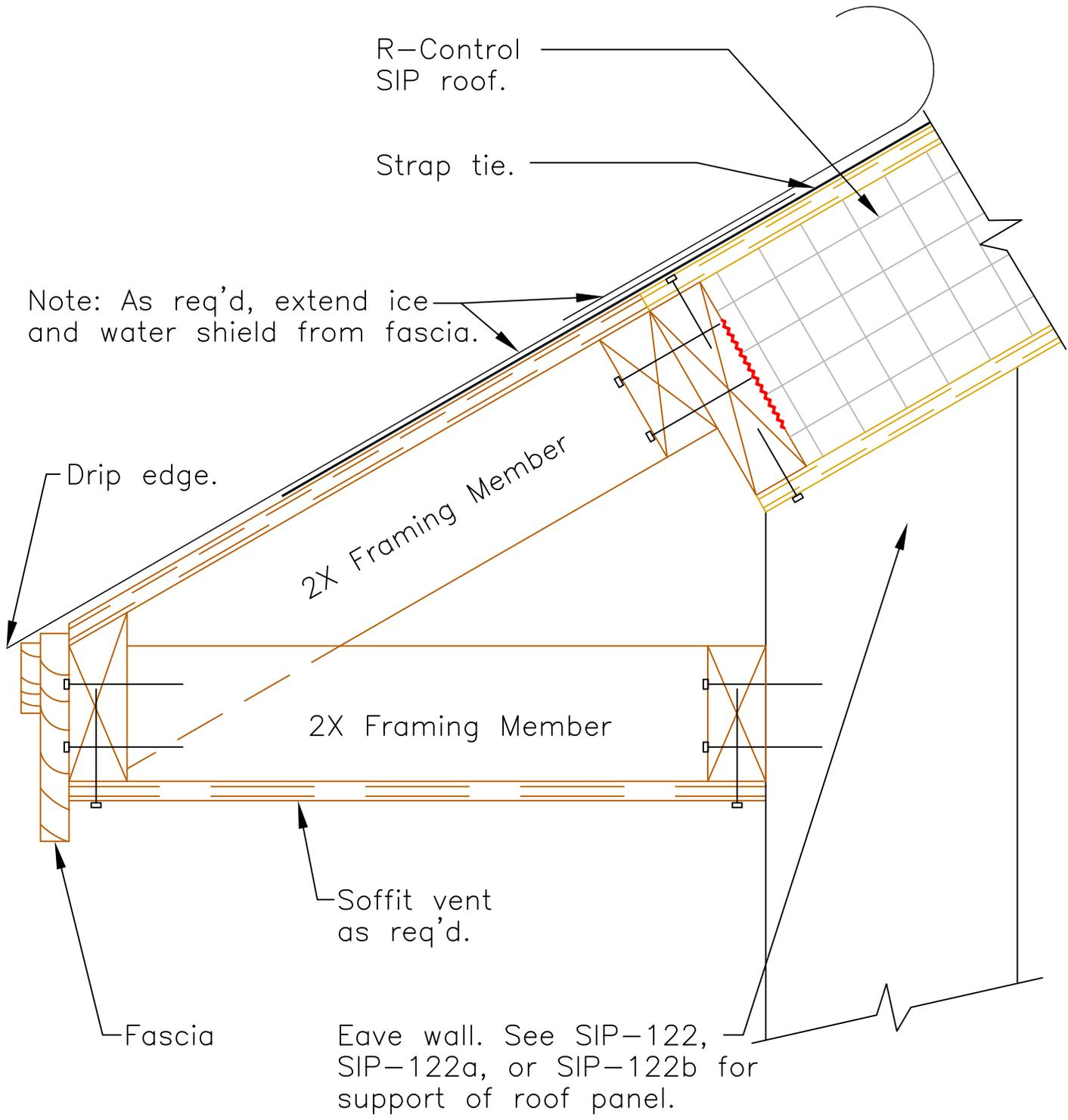
Note: As req'd, extend ice and water shield from fascia.
