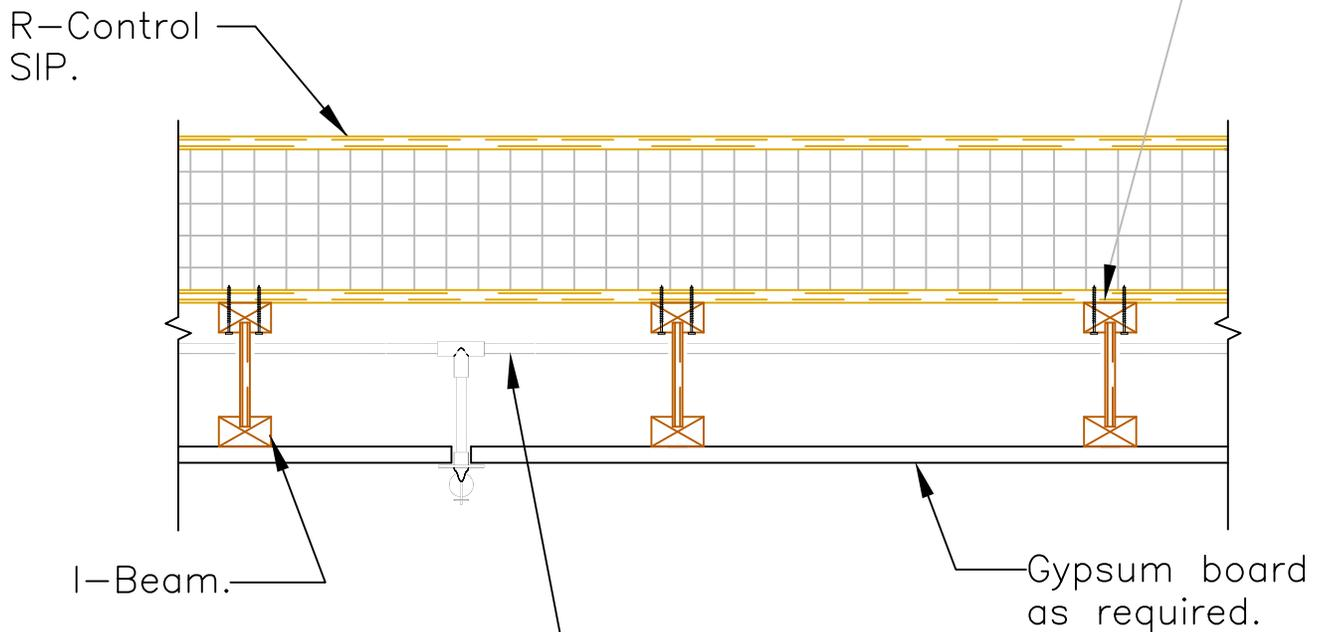
Note: I-Beam to be sized as required for cavity depth.
