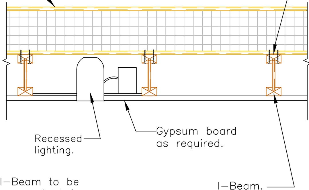
Note: I-Beam to be sized as required for cavity depth.
