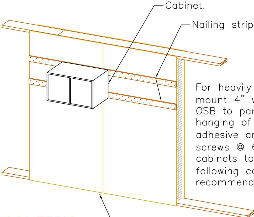
For heavily loaded cabinets mount 4" wide strips of OSB to panels prior to hanging of cabinet. Use adhesive and 2 rows of #8 screws @ 6" o.c. Fasten cabinets to nailing strips following cabinet manufacturer's recommendations.
