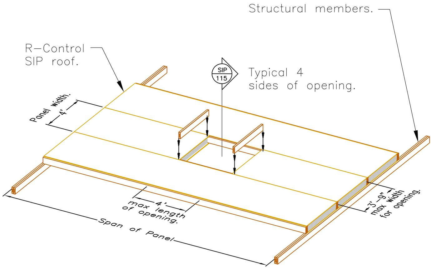
Note: For openings bigger in size than shown above or for openings that cut through splines, provide additional framing to support panel edges. This additional framing is to be located under the panels and framed into the main structural members.
