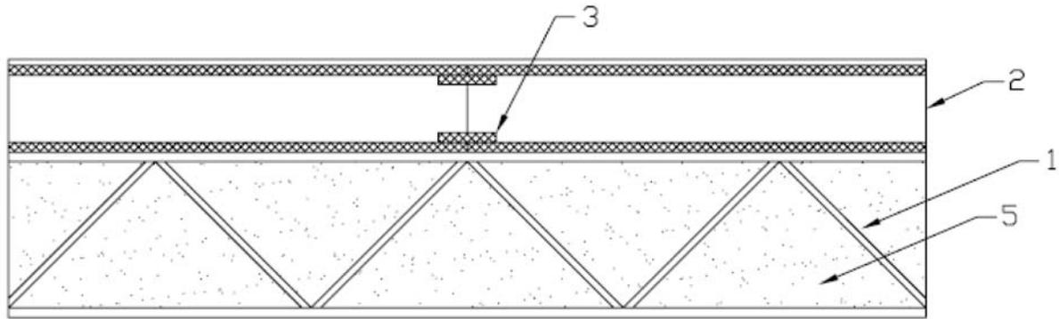
1. Steel Joist - Type 10K1 min size spaced in accordance with manufacturer's installation specifications.
