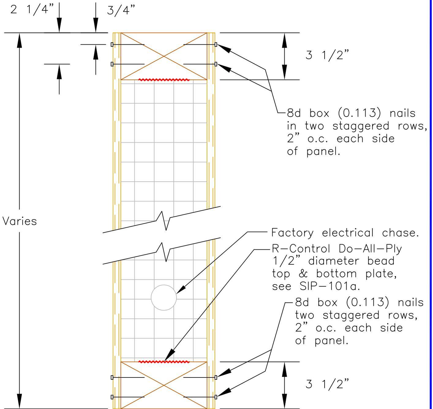
NOTE: OSB facings must be fully supported by foundation system.
