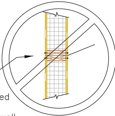
Don't have additional cap plate less than full panel width.
