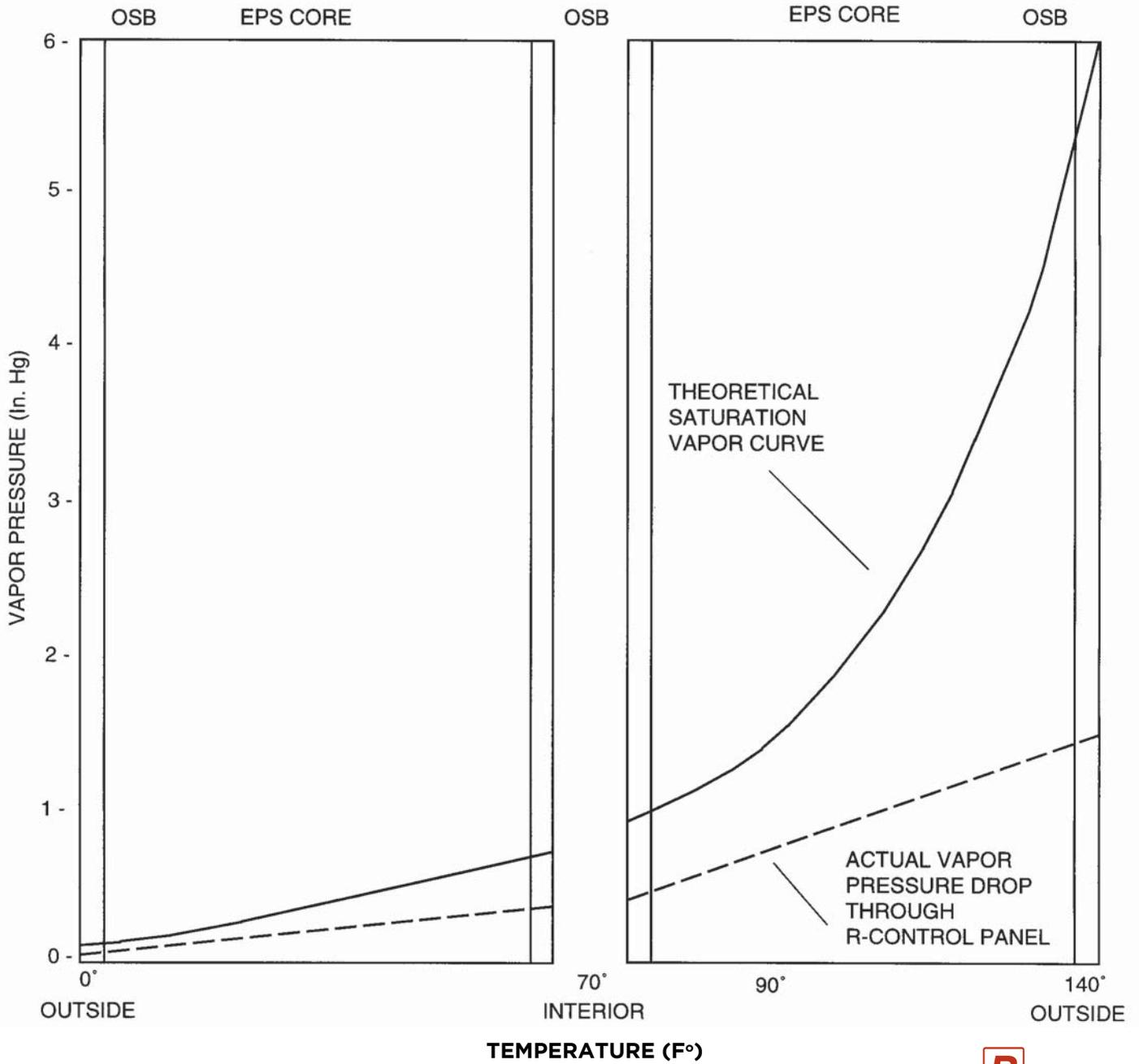
NOTE: Since vapor pressure through the R-Control SIP does not exceed saturation curve, condensation does not occur.
