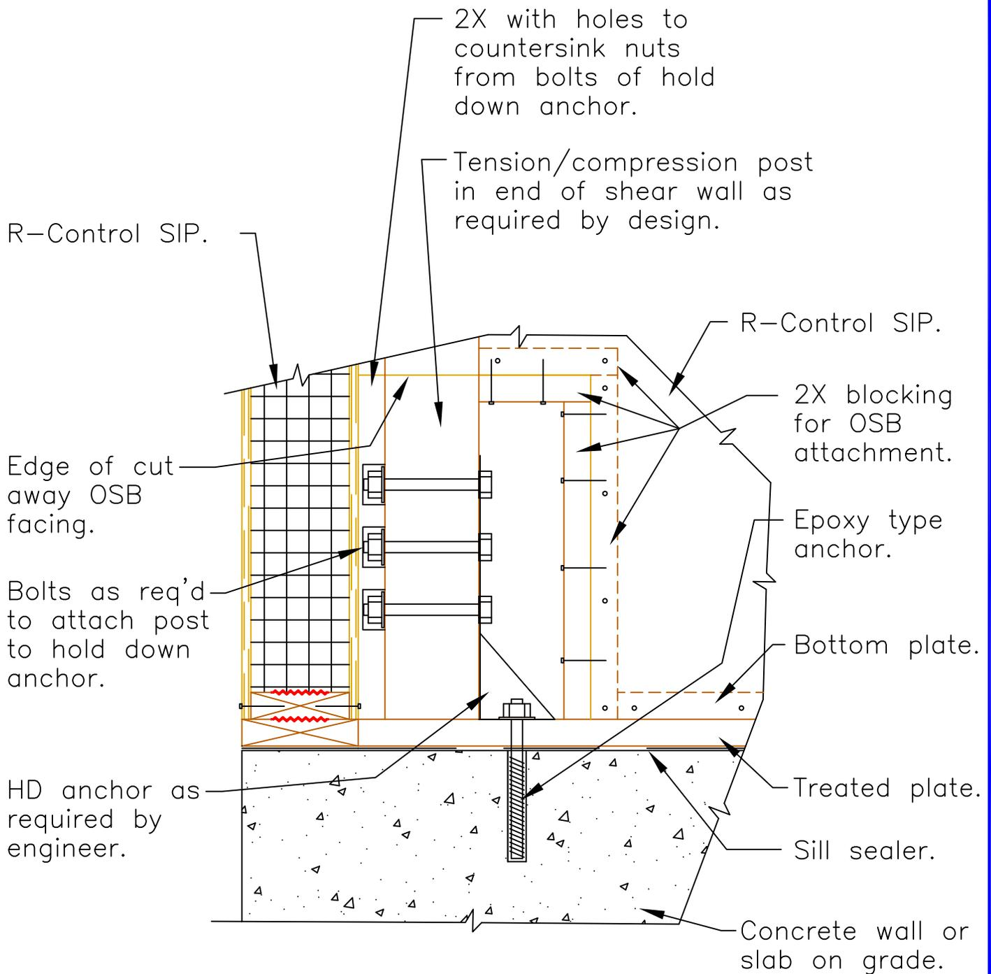
Note: Cut panel facings to place HD type anchor, post and 2X plate. Use expanding foam to fill in area around hold down anchor. Insulate cavity with low expanding foam. Replace OSB facing and nail to 2X blocking.
