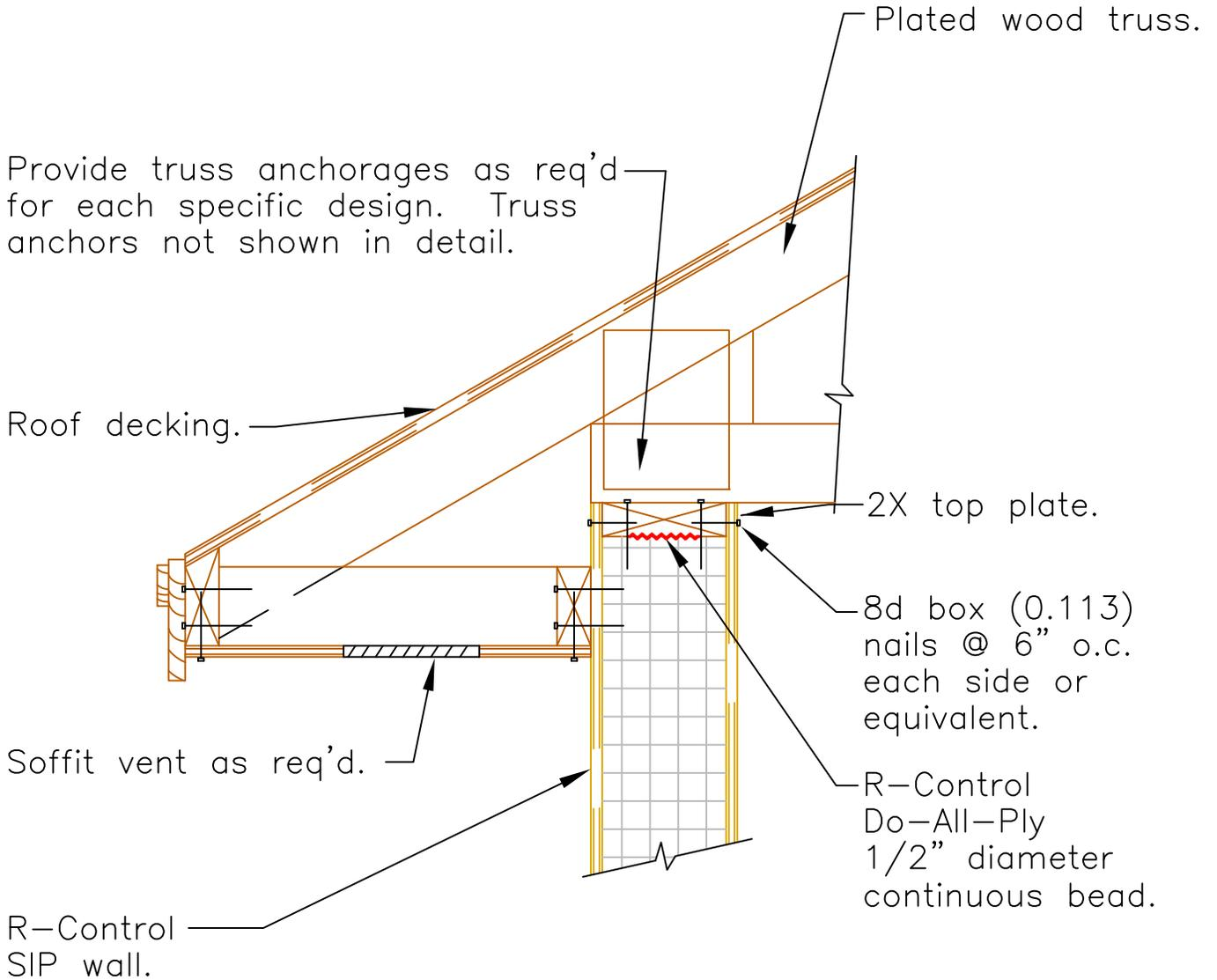
Note: Design member sizes and connections as req'd for each condition and/or project.
