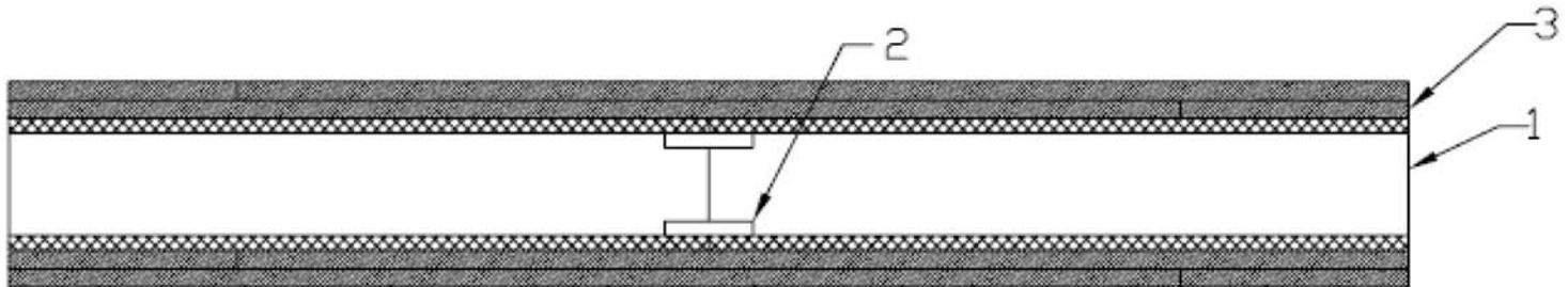
1. Panels - R-Control SIPs consisting of a polystyrene foamed plastic core faced on both surfaces with min 7/16 in. thick oriented strand board. Min 3-3/8 in. thick polystyrene core. R-Control SIPs loaded to 1800 lb. per linear foot.
