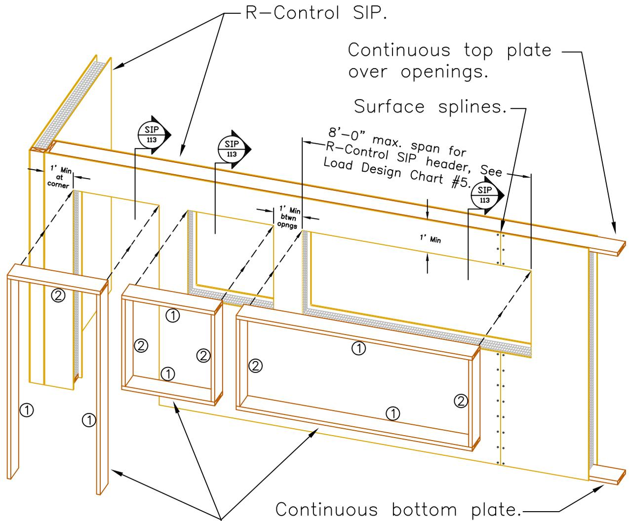
2X plating around window and door openings. Numbers indicate sequencing for installation. Refer to SIP-115 for connection of 2X's to OSB facings.
