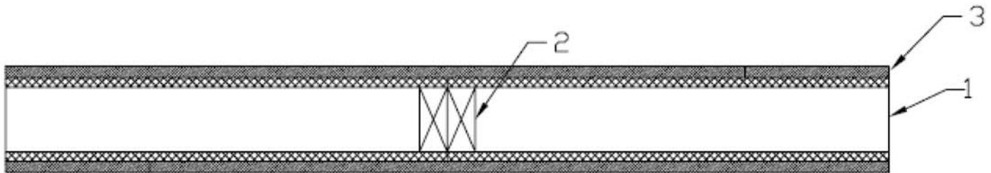
1. Panels - R-Control SIPs consisting of a polystyrene foamed plastic core faced on both surfaces with min 7/16 in. thick oriented strand board. Min 5-3/8 in. thick polystyrene core. R-Control SIPs loaded to 1800 lb. per linear foot.
