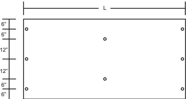
*Connection patterns for two span condition*
