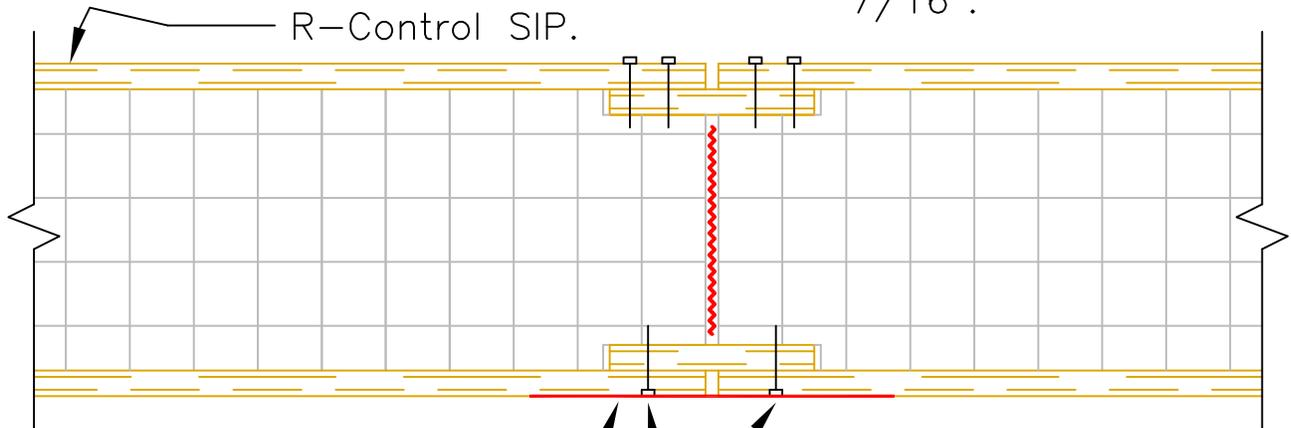
SIP Tape or equivalent vapor retarder located interior or exterior per climate conditions or code requirement.
