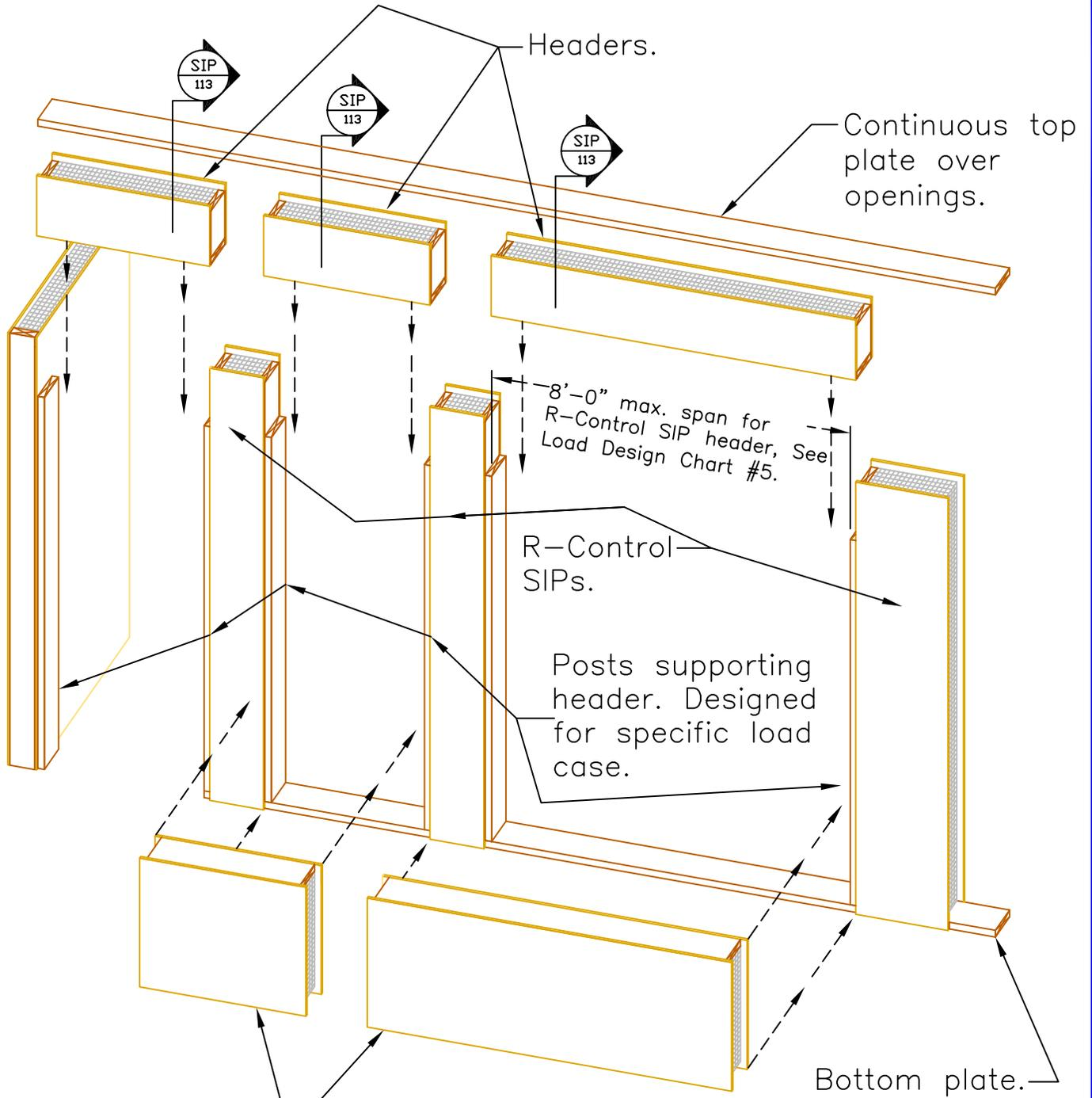
R-Control SIP infill below window openings, install prior to headers.
